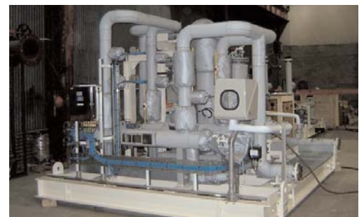
Ulva Shield, applied to vendor skid
