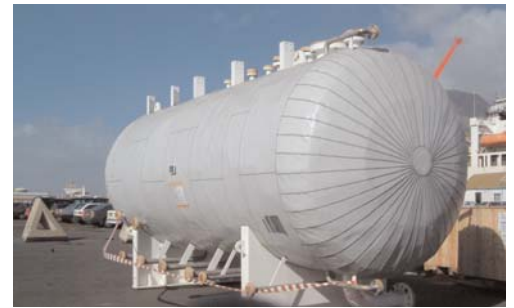
Ulva Shield applied to vessel at vendor fabrication yard prior to transit
